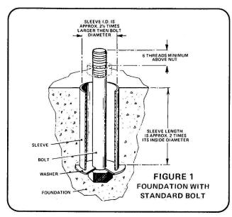
sleeve that is approximately 2- 1/2 times the bolt diameter of the sleeve. When using a standard bolt (figure 1) a washer should be used to support the head of the bolt in the sleeve. After the concrete foundation has been poured, the pipe sleeve remains in place allowing for alignment with the holes in the motor feet.
